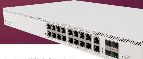
There are 17 Gigabit Ethernet ports: #1 - #8 Gigabit Ethernet ports with 802.3af/at PoE-out, #9 - #16 802.bt PoE++ ports, and an extra Gigabit Ethernet port for management purposes. There's also a console port, and four 10G SFP+ fiber ports for uplink.
