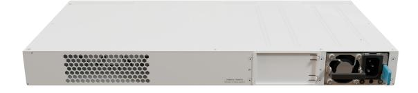
Unlike our previous "802.3af/at/bt-compatible" products, **this is our first PoE switch with full implementation of the 802.3af/at/bt standard**. It is designed to power devices with Isolated Power Delivery. While it can also power low-voltage and "802.3af/at/bt-compatible" Power Delivery devices, **you must avoid specific grounding scenarios**. Please refer to the official <u>Help page</u>.
