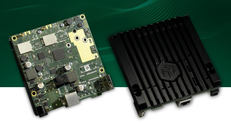
The powerful Wi-Fi 6 radio with MMCX connectors enables further customization: add a HGO-antenna-OUT and you've got yourself an excellent omnidirectional AP... or try the mANT30 PA antenna to create a powerful long-range point-to-point link!
