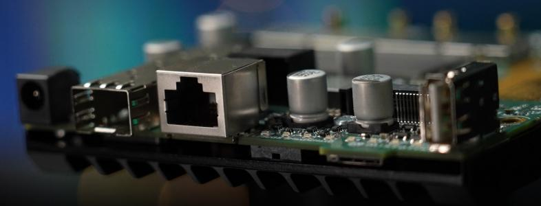
This modular board features a modern Qualcomm Maple CPU based on the ARM architecture, a USB port for extra storage or other needs, **Gigabit Ethernet with PoE-in, 2.5 Gigabit SFP** for fiber connectivity, and a **free miniPCle slot** that allows further customization. You could, for example, add an LTE modem for a mobile internet backup – we've added a NanoSIM slot on the bottom! But there are other options, like adding a gateway for LoRa IoT setups, such as our R11e-LR8!
