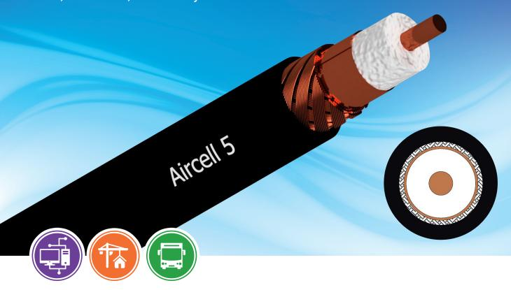
Aircell 5 is a flexible and thin coaxial cable with a 5 mm outer diameter designed for the frequency range from DC to 10 GHz. Its low-loss characteristics in relation to its diameter and compatibility with standard RG 58 connectors make it the preferred choice not only for Wireless LAN applications but also for general RF communications.
